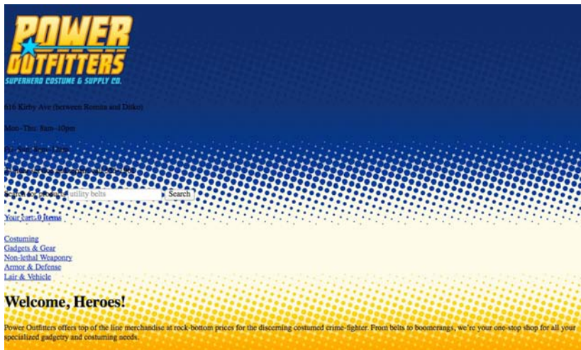
Figure 10-5. Our comic-inspired, dot-patterned background, accomplished with two images in two positions, filling the html element.
