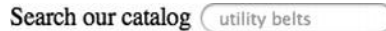
Figure 8-3. How the search field appears in Safari, including placeholder text. Safari styles search inputs with rounded ends by default, in keeping with Apple's general style for search boxes on OS X, but other browsers will differ.
